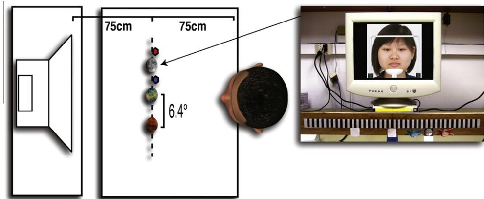
**Fig. 2.** Schematic representation of the apparatus used in Experiment 1. The photograph displays the configuration of targets and fixation positions for a block during which the observer judged whether the model was looking to the right or left of a target  $6.4^\circ$  to the right of the midline. The arrow shows the relevant target in the version of the apparatus depicted in the accompanying photograph.
